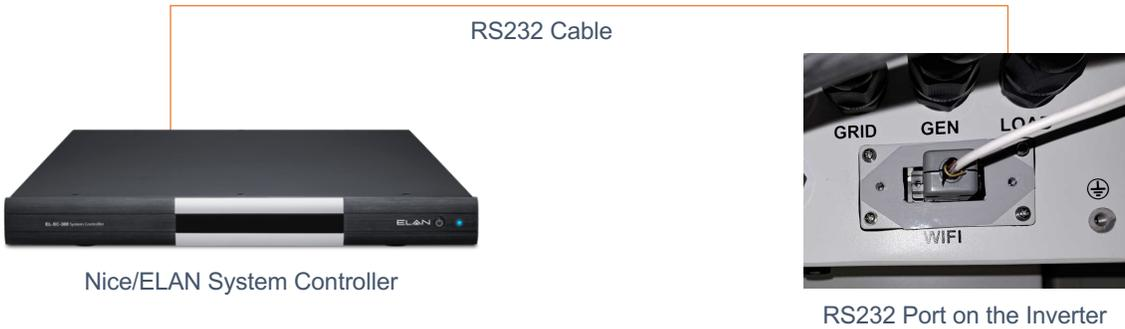
The ELAN controller can be connected to your inverter using an internal RS485 Port on your inverter using an RS232/RS485 converter. Most Synsynk/Deye inverters use pins 7(+) and 8(-) on the RJ45 socket. RS485 ports on ELAN controllers are not compatible with this driver because there is no supported method of configuring them as RS485 half duplex.
