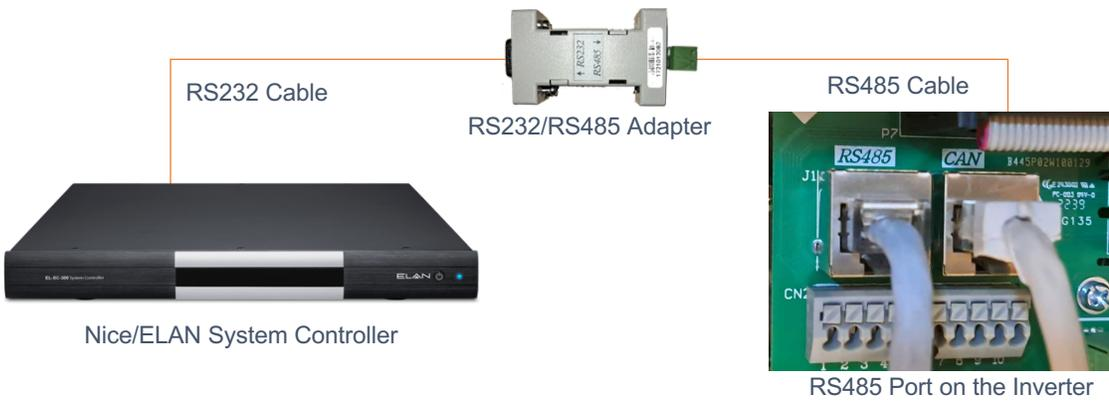
Virtual interfaces supported by ELAN controllers, such as the Global Cachè serial ports, can also be used. Serial ports must be configured at 9600 baud, 1 stop bit, and no parity.
